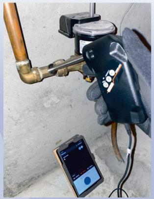
PERIJA Mini Vpro is a **Leak Judgment Instrument & Acoustic Digital Sound Detector Electronic Listening Stick System** with **Automatic Water Leakage Judgment Mode**, well-suited for water leak surveying on pipes for **Service Lines between homes**. It is a smart and sensitive sound detector that is equipped with an internal piezo electric sensor in an extremely small size.
